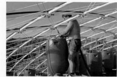
6.20 Water barrels representing partial snow load
