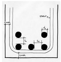
Horizontal Spacing in Beams
