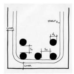
Horizontal Spacing in Beams
