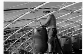
6.20 Water barrels representing partial snow load
