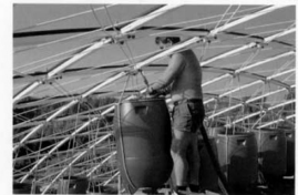
6.20 Water barrels representing partial snow load
