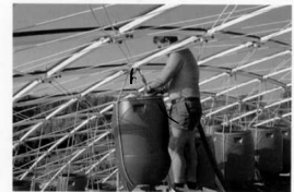
6.20 Water barrels representing partial snow load
